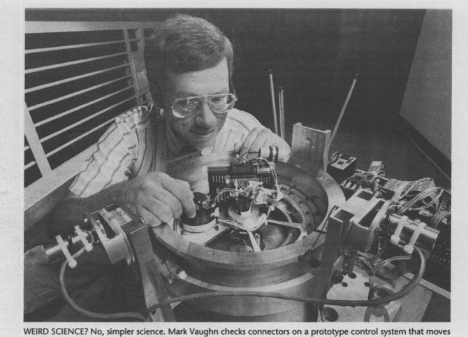
weights around a circular rim to reorient a rocket flight or satellite orbit without use of jets or jet fuel.
